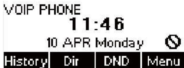
Figure 56 - DND Enabled on All Lines
